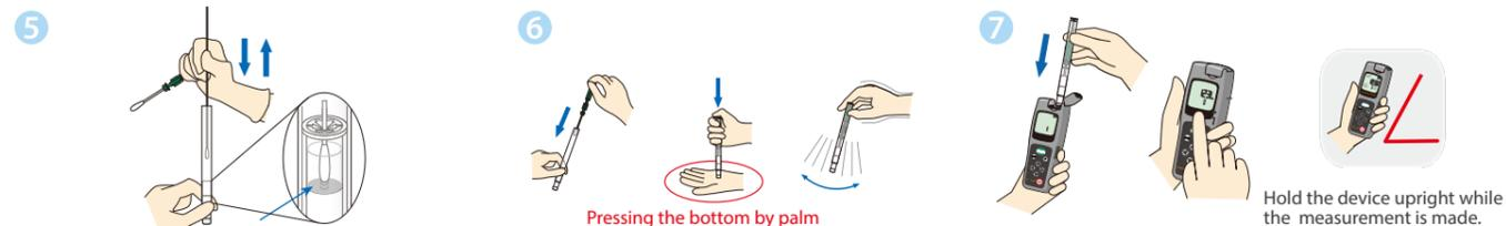
Insert the LuciSwab into the main body of the LuciPac, then wash LuciSwab in releasing reagent. Be careful not to break the aluminum seal.
