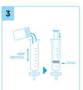
Pour water sample into syringe. Write down exact volume (approx. 50ml) to be analysed. Filter vertically water sample until you feel resistance. Stop immediately to avoid drying filter (with 10mL of air remaining).
