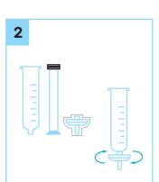
Remove syringe piston and place carefully, avoid touching black plunger. Open filter packaging (do not discard cup, this will be needed in step 4). Firmly screw syringe onto filter.
