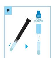
Immediately, take tube holder out of luminometer. Remove MICRO TUBE from tube holder. Add one drop of **STANDARD** (blue cap) into MICRO TUBE, without inserting nozzle of dropper bottle, to avoid contact with MICRO TUBE.
