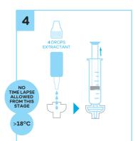
Using cup from filter packaging, place 4 drops of **EXTRACTANT** (white cap), then place filter tip at bottom of cup to draw up reagents. Maintain upward pressure on
