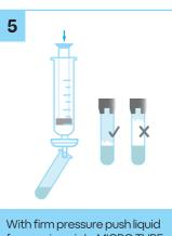
from syringe into MICRO TUBE until white foam appears. Stop pressure as soon as foam appears to avoid creating «stopper» in upper part of tube.
