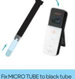
holder. Place in luminometer and press the ENTER button to start measurement. Write down the R1 result (in RLU).
