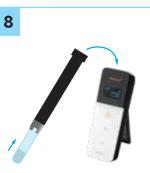
Fix MICRO TUBE to tube holder and homogenize mix by tapping MICRO TUBE on a flat surface. Place tubeholder in the luminometer and press Enter. Write down R2 result (in RLU).
